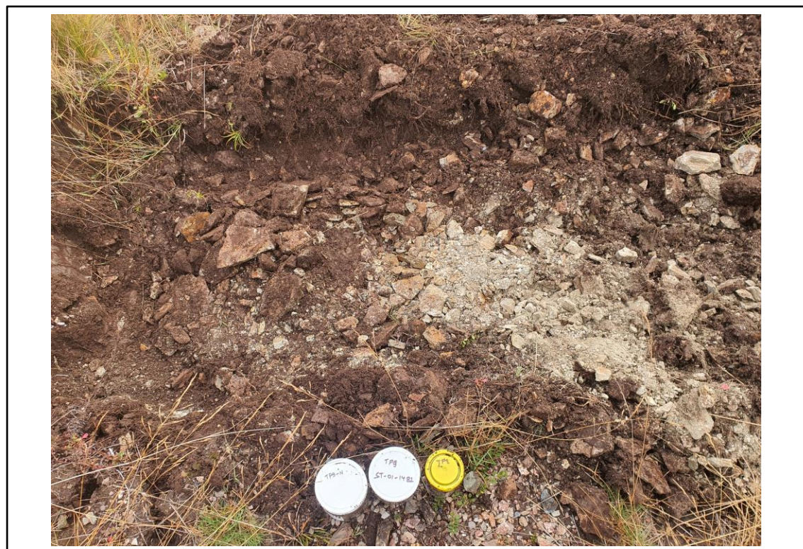
Photo.6. Representative photo of soil and gravel observed at test pit TP9.
