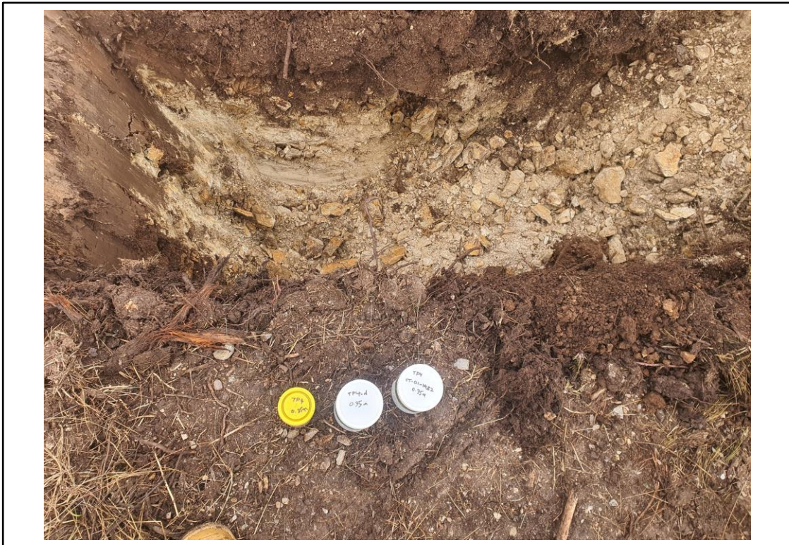
Photo.5. Representative photo of soils and natural rock encountered at test pit TP4.
