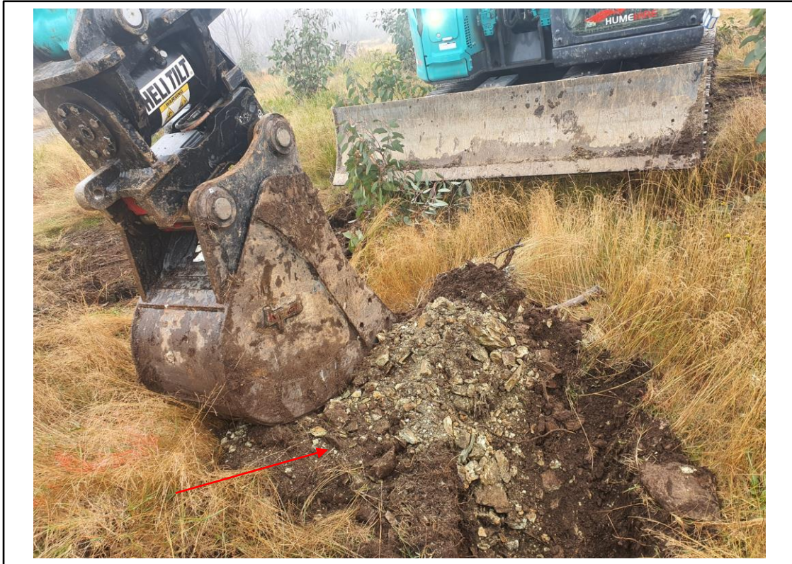
Photo.1. Representative photo of the soils onsite (Gravelly Clay Silt)
