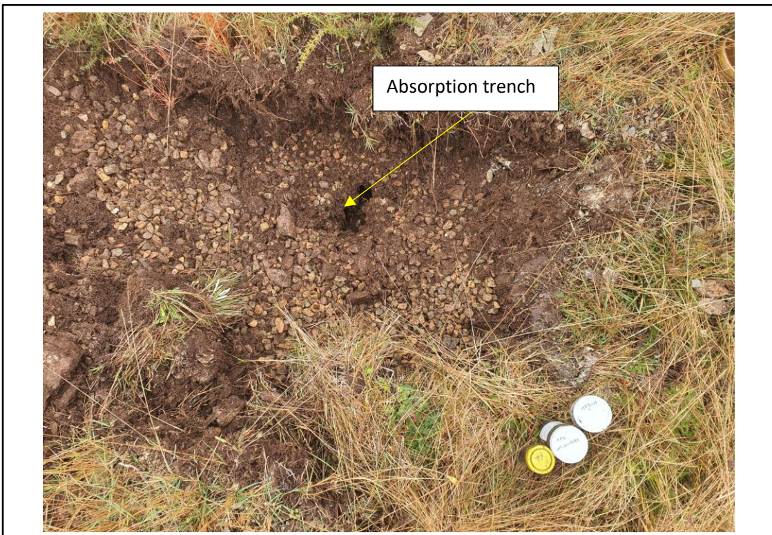
Photo.4. Representative photo of materials observed at test pit TP3 where the sub-surface trench was observed.
