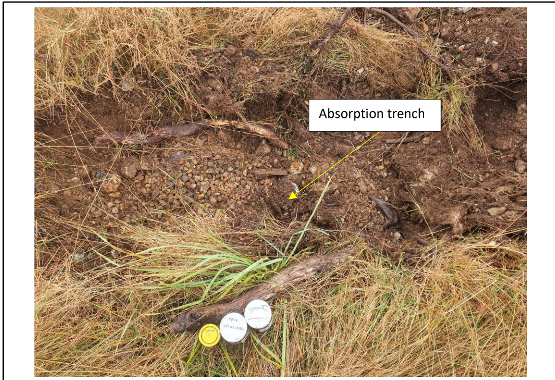
Photo.7. Representative photo of materials observed at test pit TP3 where the sub-surface trench was observed.
